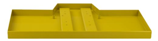
Made of 1/16" (1.5mm) thick sheet steel, powder-coated. Secure stand due to drill holes for fastening to a work surface (the use of steel sleeves keeps the tray tightly sealed). 27 1/2" x 16/12" x 1 37/64" (L 700mm, W 420mm, H 40mm).
