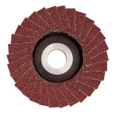
For grinding tempered cast iron, cast iron, stainless steel, non-ferrous metals, wood and plastic. For producing smooth, fine surfaces. For intermediate and fine sanding. Ø 50mm. With 10mm bore.
