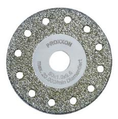
For cutting, grinding, and roughing of hard materials such as glass, porcelain, ceramics and stone. Less heating up due to cooling holes.  $\emptyset$  50 x 1mm. With 10mm bore.
