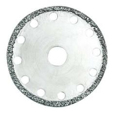
For fine cuts in hard materials such as glass, porcelain, ceramics and stone. Less heating up due to cooling holes.  $\emptyset$  50 x 0.6mm. With 10mm bore.
