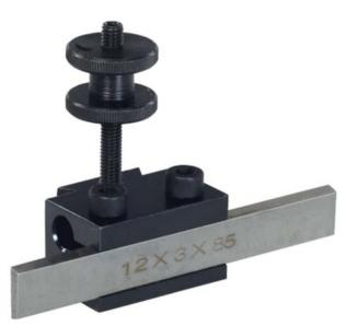
Used in the PD 250/E quick change system. Used to part stock and cut slots. The 12 x 3 x 85mm HSS tool contains cobalt. Spare tools available under NO 24 554.
