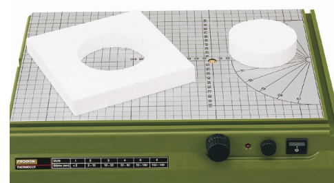
Crosscuts are achieved by means of a simple, yet efficient solution: secure drawing-pin to table with tape, it serves as a fixed center.
